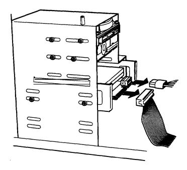
2. Remove the four screws (two on each side) securing the drive to the drive bay. Then slide the drive out through the front of the bay.
